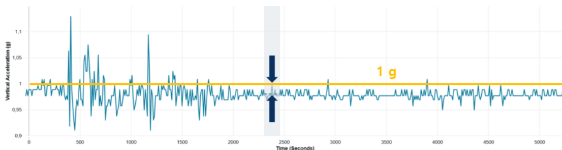
Figure 11 - Illustration of the bias in the vertical acceleration parameter for a flight. Grey band corresponds to the window in which flight is considered stable
